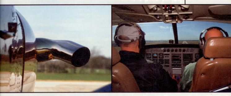
**TRAILING-EDGE** lift-augmenting devices are part of the payload extender package on the 2002 model 208A flown for this article (below left). Larger air intake ductwork (below) is another feature of the conversion, as is an oil quantity sight gauge (right) that replaces the stock engine's dipstick.
